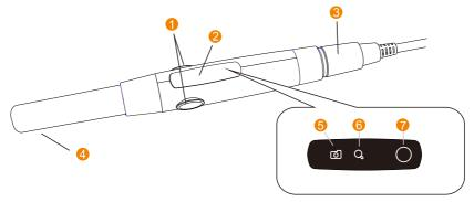
0 Image capture button/ 0 User interface/ 0 USB Plug/ 0 Camera lens/ 0 Camera status indicator/ 0 Macro button
