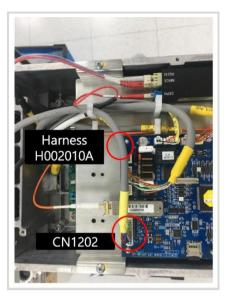
4. Connect H002010A of the CEPH unit to CN1202 of the MCU board.
