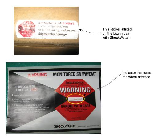
Please check the color of ShockWatch on the carton. Even if the indicator is red, it does not necessarily mean that the unit had been damaged. However, immediately contact the Delivery Company, agent, or VATECH.
