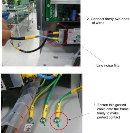
2. Connect firmly two ends of wires
