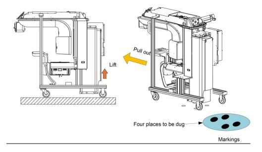
K. Drill four floor holes marked at the **step K** where the equipment is to be installed, as stated in the following figure.
