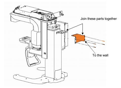
3. The following figure shows the 3-dimensional view after the floor anchors and wall mount bracket are installed.
