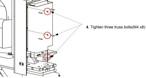
3.4 Assembling the power board bracket
