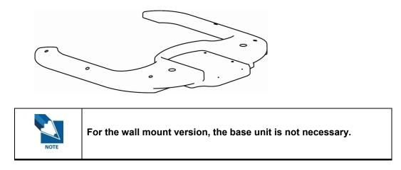
D. Push the base unit through the space under the equipment, as shown in the following figure.
