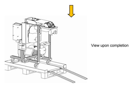
4. Unload the equipment from the crate and move it near the installation site.
