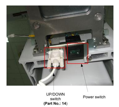
1. Connect the UP/DOWN switch, as shown in left figure
