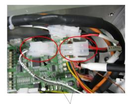
1. Connect the cables named CEPH 24V
