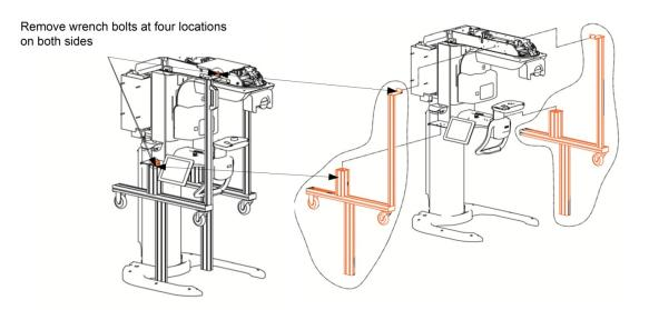
P. Finally separate the sub-plate from the equipment, as illustrated in the following figure.
