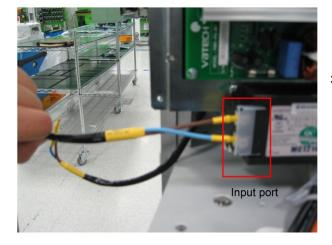
3. Connect the other end of cable **18A** With the input port
