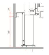
3. Mark four hole positions on the wall to where the bolts are to be anchored.
