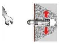
5. Attach and tighten the wall bracket (**Part No. 40**) to the wall, with the anchor bolts (**M8**: **Part No.:40**).
