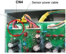
**Work**: connect the sensor power cable to the CN4
