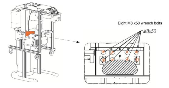
O. After raising the column up by about 5 cm, remove the wrench bolts on both sides to separate the support frames (colored) from the equipment.
