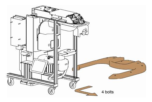
E. Slide (push) the base unit to the rear close enough until four holes are matched, as shown in the figure.
