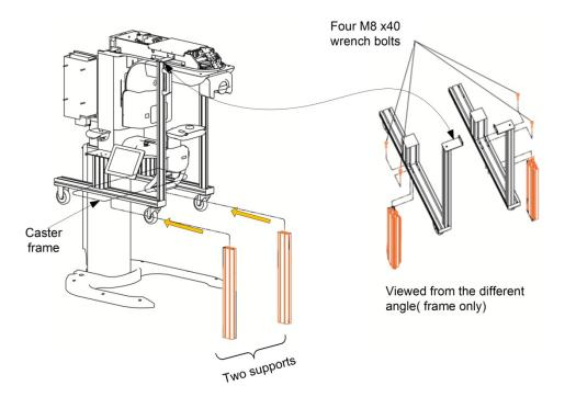
L. Remove two transportation bolts that hold the rotating unit and column in position—installed to prevent the equipment from tipping forward, due to the center of gravity.
