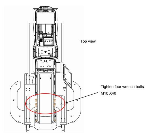
The following figure shows the resulting assembly of the base unit with the main unit.
