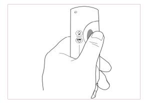
Adjust the height of the unit to fit the patient. Press the Up & Down button of the Column switch to adjust the carriage until the ear rods are properly positioned adjacent to the patient's ears.
