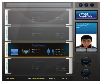
The above image shows the main window of the imaging software. Its sole purpose is to control the equipment and acquire images. By default, Standard Panoramic mode is activated.
